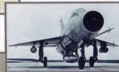
▲ Design limitations Compared to Western fighters of the period, the MiG-21 was small, sleek and simple. This resulted in limited avionics and armament, and the early variants were barely acceptable as frontline fighters.
